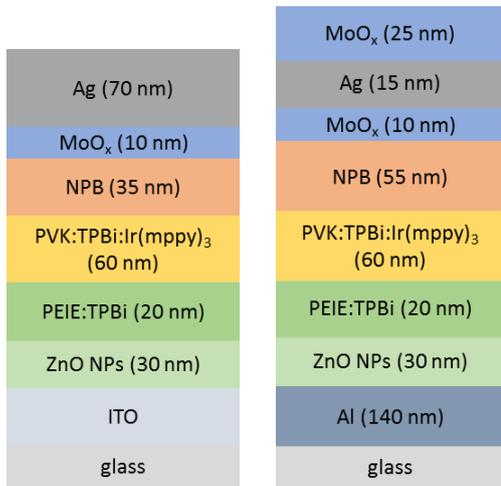
Figure 1. Bottom-emitting (left) and top-emitting (right) OLEDs based on iridium complex.
