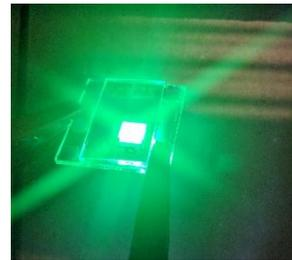
Figure 2. Top-emitting OLED based on iridium complex.
