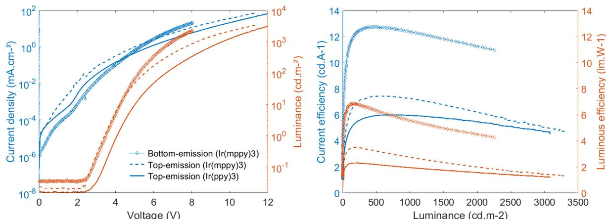
Figure 3. Current density-voltage-luminance characteristics, current efficiency and luminous efficiency of solution-processed bottom-emitting PhOLED and top-emitting PhOLED, based on Ir(mppy)<sub>3</sub> and Ir(pppy)<sub>3</sub>.
